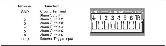
Figure 3-9. Rear-Panel Alarm Outputs
