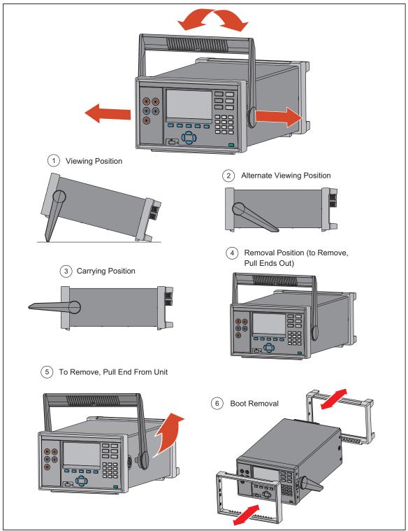
Figure 2-3. Handle Positions and Boot Removal
