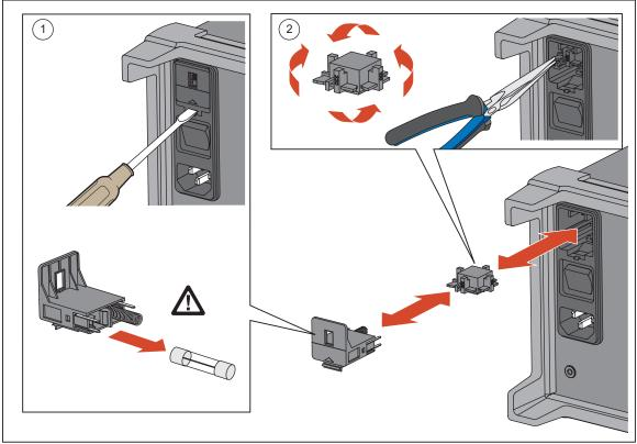
Figure 2-1. Fuse Replacement and Line-Voltage Selection
