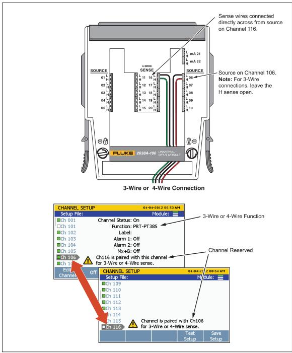
Figure 3-2. 3-Wire and 4-Wire Channel Reservation
