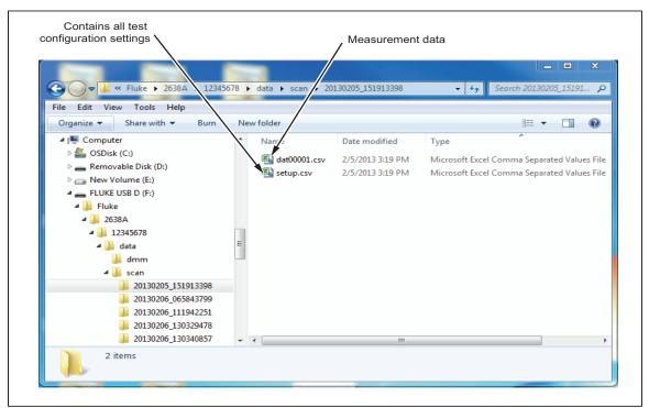
Figure 4-8. Setup.csv and Dat00001.csv Files
