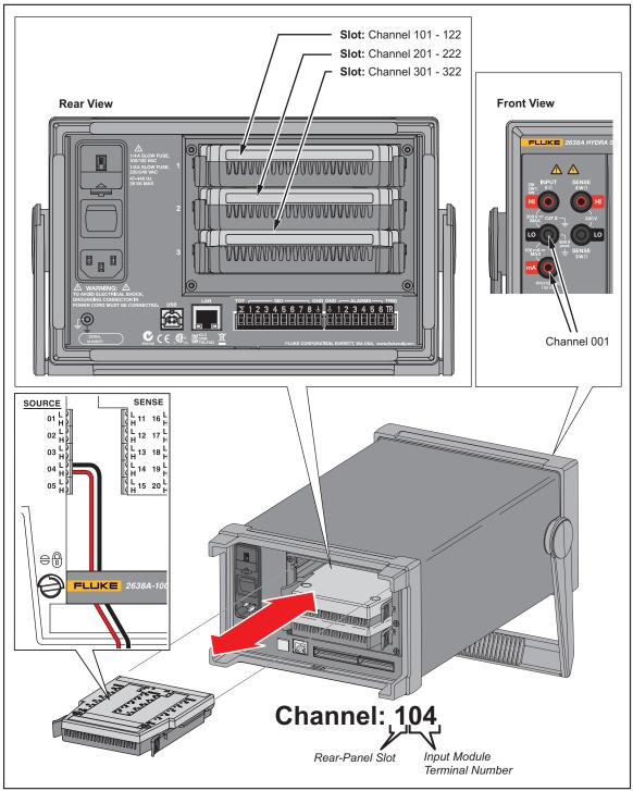
Figure 3-4. Example Channel Assignment
