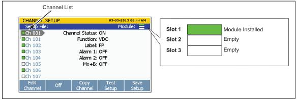
Figure 2-5. Module Indicator Example
