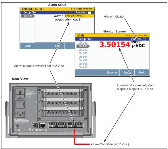
Figure 3-10. Alarm Output Example
