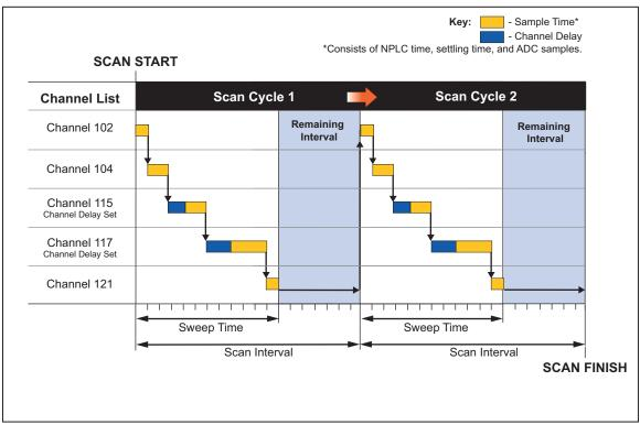
Figure 4-2. Illustration of a Scan Sweep
