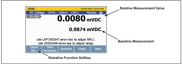
Figure 5-3. Relative Measurement
