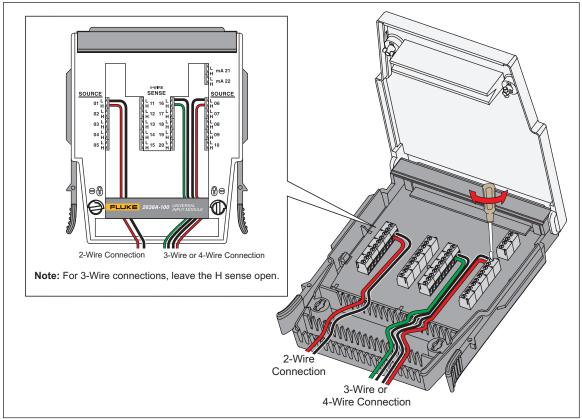
Figure 3-1. 2-Wire, 3-Wire, and 4-Wire Example Connections
