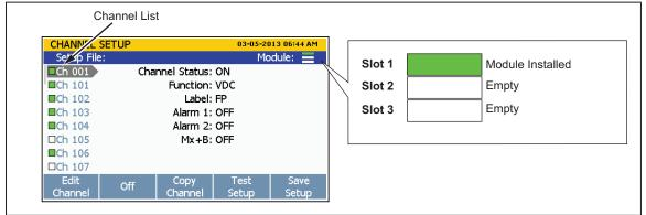
Figure 3-3. Module Indicator (Input Module Installed Shown)
