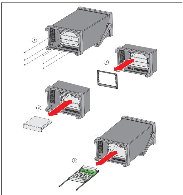
Figure 2-6. Relay Card Installation
